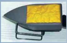
Fig. 3C Temperature test at approx 150°C
